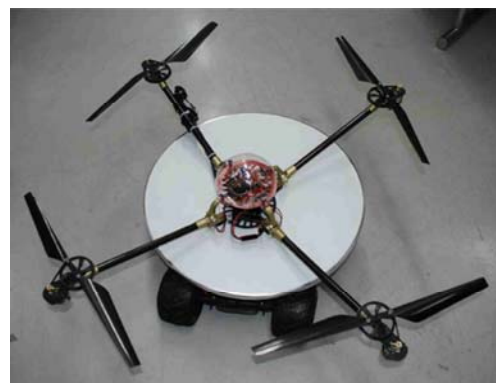
Fig. 1. Quadrotor helicopter on a landing pad under consideration.
