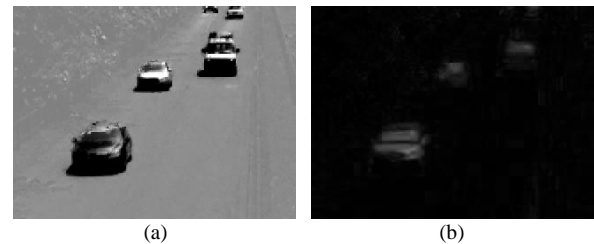
Fig. 7. Brightness variation and chromaticity variation extracted from the same images as in Fig. 6. The brightness variation is added by 128 and shown in (a), and the chromaticity variation is multiplied by 2 and shown in (b).
